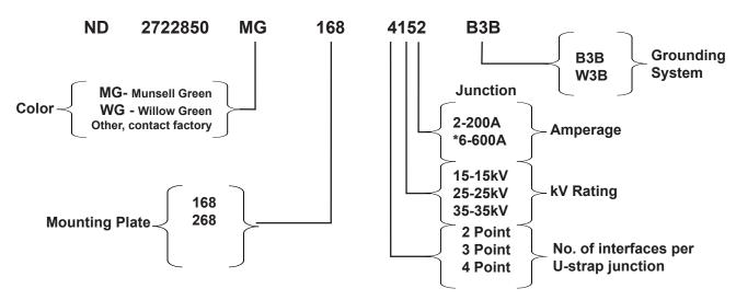
\*This cabinet will accommodate 15-35kV, 200 & 600Amp junctions with U-straps. It will accommodate 200Amp taps off the 600Amp deadbreak junction. It will also accommodate Cooper 35kV 200/600Amp loadbreak junctions.
